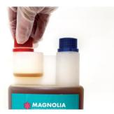
6. Unscrew and remove the red cap fully and pour the solution into the Pulse Cleaner Bucket making sure that no extra solution travels up the pipe from the main bottle.
